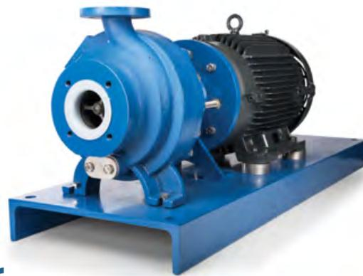
“The original pumps lasted a mere four to five months before the seals and the impellers failed.” Switching from the sealed pump technology to magnetic coupling eliminated the issues with worn seals and the inevitable leaks they caused.
