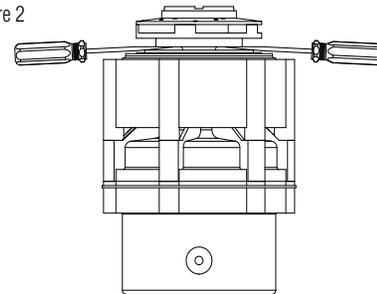
7. Remove the diffuser assembly (item 22) and the diffuser O-ring (item 21) from the top of the 2nd stage impeller housing (item 20). Remove the 2nd stage impeller housing (item 20), the housing O-ring (item 17), and the 2nd stage impeller assembly (items 18 & 19) from the barrier/column-housing adapter (item 16).
