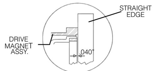
**⚠ CAUTION:** Do not operate/test the motor with the drive magnet assembly exposed.
